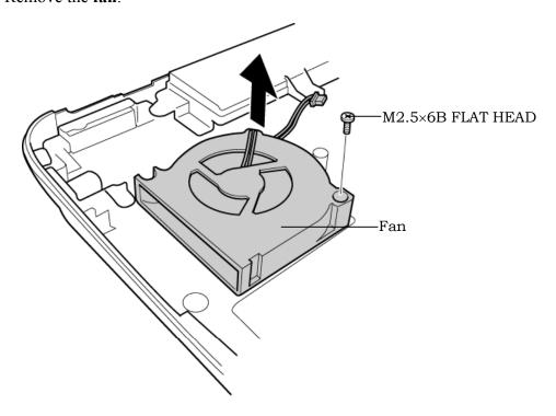
Figure 4-33 Removing the fan
